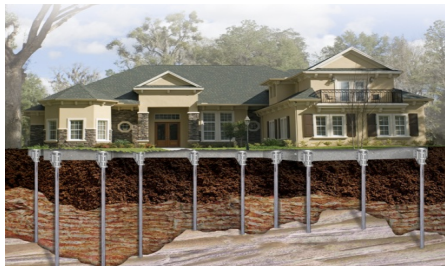
Home with perimeter underpins that rest on limestone and were installed to support load-bearing members and transfer the load to solid, stable soils or rock.
